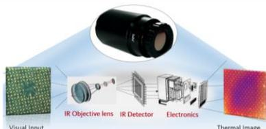
Figure 2. Schematic diagram of thermal imaging principle
