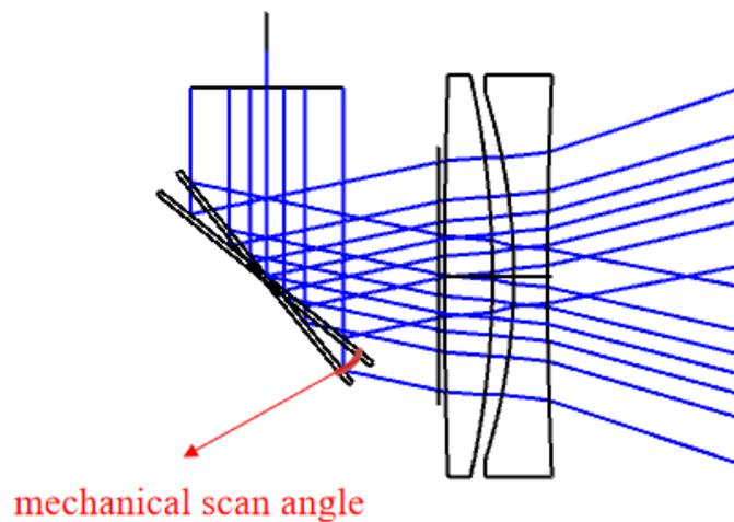
We use two mechanical scanning mirrors as Mirror X angle and Mirror Y respectively, then the relationship between them and the optical scanning angle is:
