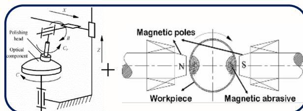
Figure 1. Two-step process of super-polishing technique
