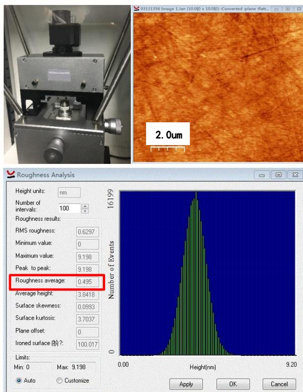
Figure 2. Atomic force microscope and surface roughness measurement.
