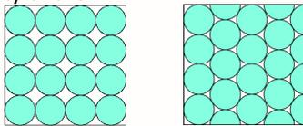
Figure 1. Square/hexagonal arrangement pattern
