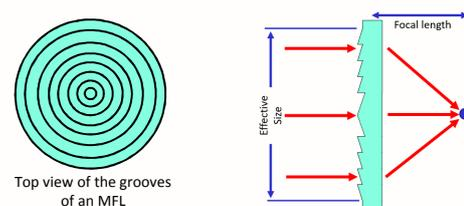
Figure 5. MFL lens causing rays to focus
