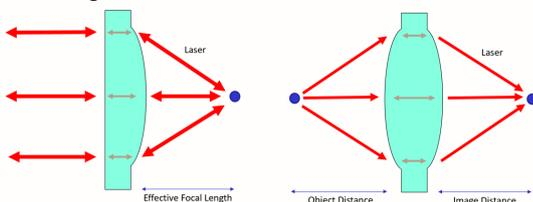
Figure 3. Ray diagram of single/dual surface lenslet
