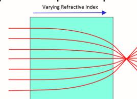
Figure 4. GRIN lens causing rays of light to bend within
