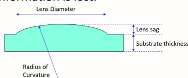
Figure 2. Parameters of a conventional lenslet
