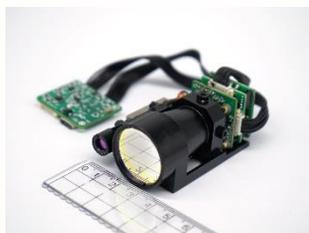
Figure 1. Image of Laser Rangefinder
