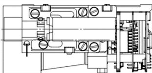
Figure 2. Outline of Laser Rangefinder
