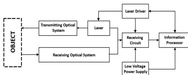
Figure 2. Laser Rangefinder Operational Layout
