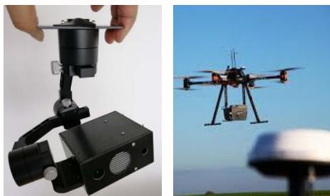
Figure 1. A prototype of compact laser dazzler
