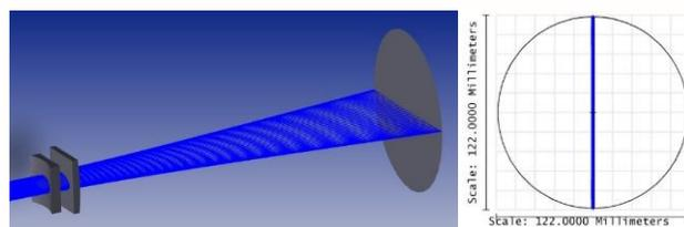
Figure 4. Design of high-aspect-ratio line beam at 193nm
