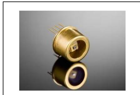
SAP500 series is based on a reach-through structure featuring excellent quantum efficiency, extremely low noise, and low dark current. To detect individual photons, the avalanche photodiode is operated in Geiger mode; it is operated at a voltage above the breakdown voltage,  $V_R > V_{BR}$ . The component has an active area of 500  $\mu\text{m}$  and comes in a hermetically-sealed TO-46 housing – optional with single-stage thermoelectric cooler (TO-37) or two-stage TEC in a TO-8 housing.
